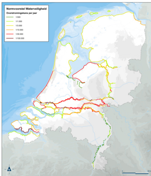
Figure 5: Proposed new safety standards for flood defenses in the Netherlands, in the form of target failure probabilities for a system (Delta program, 2014).
