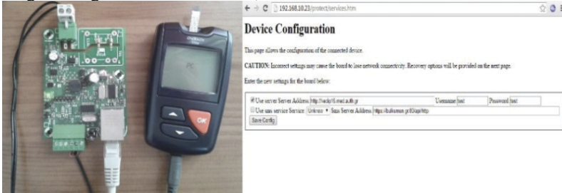
Figure 2. The glucose meter device adapted to the intermediate hardware device for XMPP compatibility (left). Configuration of XMPP server, username and password (right).
