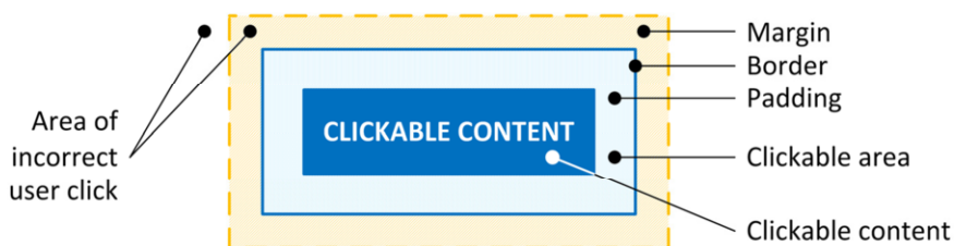
Figure 1. Box model and structure of a clickable UI element
