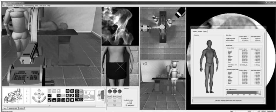
**Figure 1.** Visualization of the simulated scattered radiation and dosage values (left member of the staff) for an anterior-posterior view of the left hip joint with a tube voltage of 80kV.
