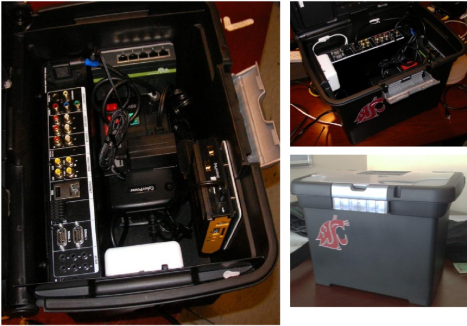
Figure 3.2. CASAS smart home components for power, networking, computation and middleware stored in a box.
