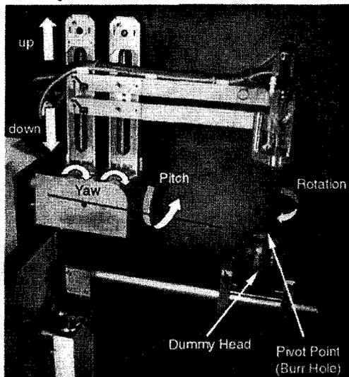
Fig. 1 NEUROBOT, the active manipulator developed within the ROBOSCOPE system. Using a standard neuro-endoscope, which is attached to the end effector, NEUROBOT can be freely moved in four degrees of freedom about a pivot point at the burr-hole. A dummy head is clamped to the robot, which is registered to the MRI data to simulate the positioning of the patient. (Courtesy of Fokker Control Systems, B.V.)
