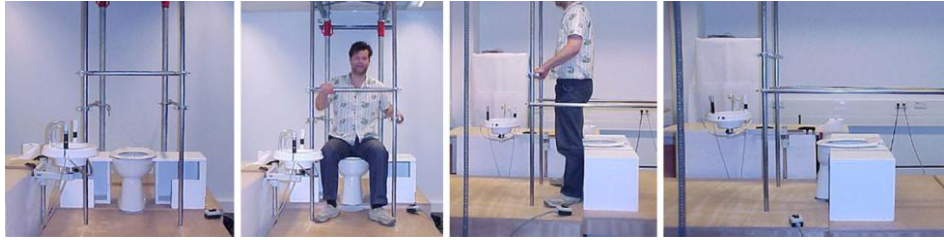
Figure 5. Laboratory test environment to determine the location for support around the toilet (Delft, NL)
