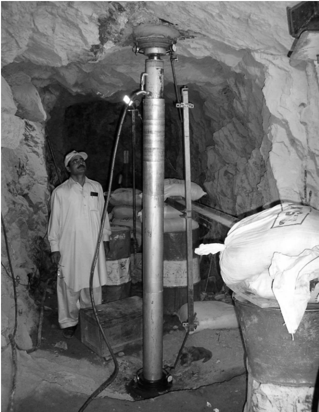
Figure 3. Vertical Rigid Plate Load Test in Adit No.1
