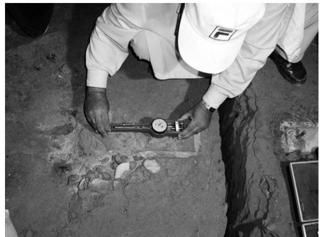
Figure 5. Measurements before inserting the Flatjack into the slot
