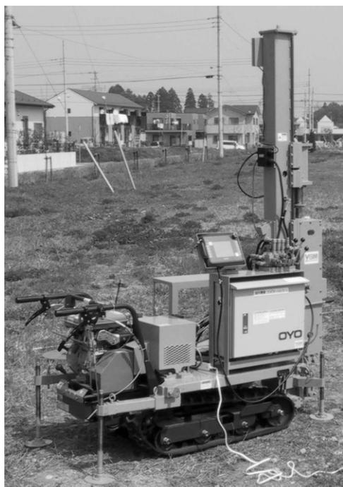
Figure 1. New combination cone penetration equipment.
