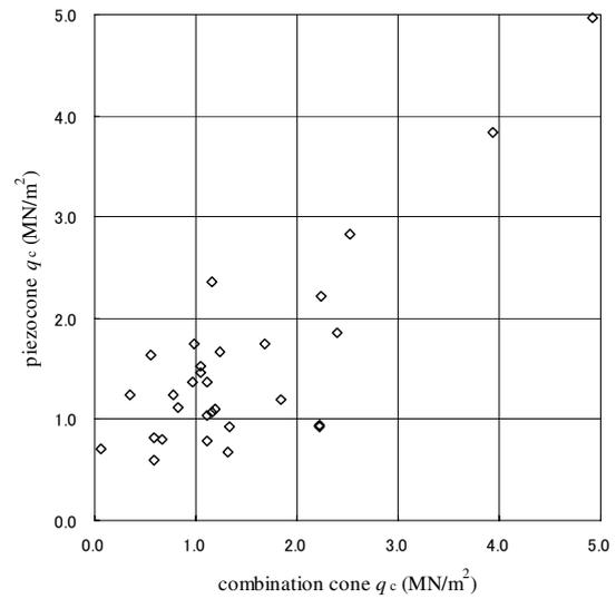
Figure 5. Relationship of  $q_c$  between combination cone and piezocone
