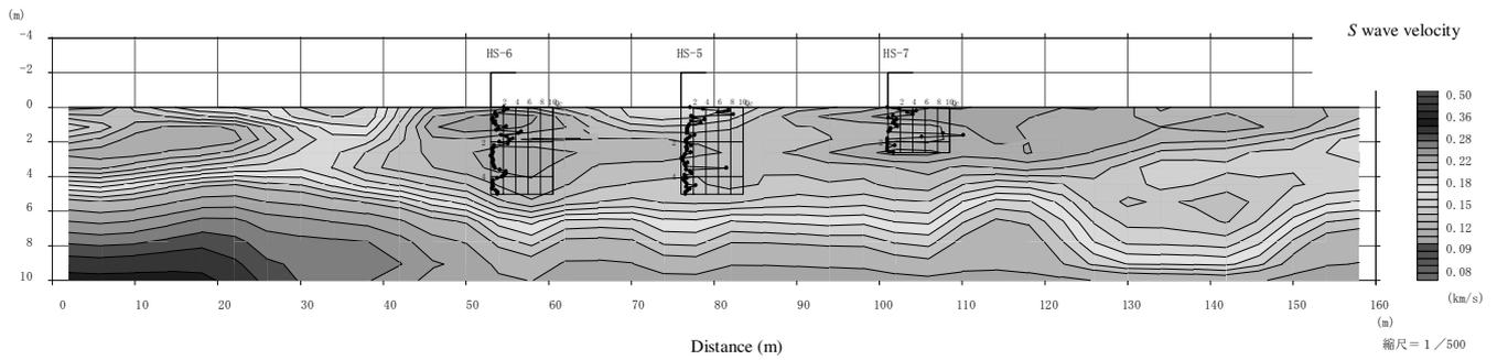
Figure 7. Cross-section of S wave velocity.
