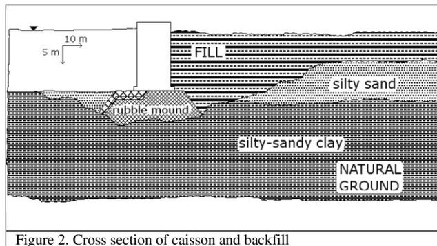
Figure 2. Cross section of caisson and backfill
