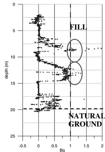
Figure 7. Application of  $B_q$  liquefaction criteria for CPTU 6a8 test. Circled points indicate potential liquefaction.
