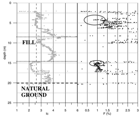
Figure 6. Application of ( $I_c$  & F) liquefaction criteria for CPTU 6a8. Circled points indicate potential liquefaction
