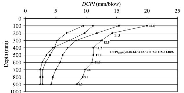
Figure 4. DCPI values obtained for different depths
