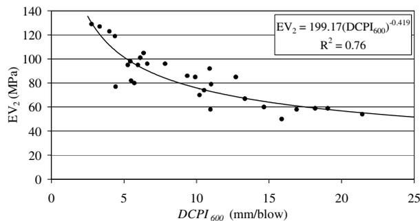
Figure 6. Relation between  $DCPI_{600}$  and  $EV_2$  for coarse-grained soils
