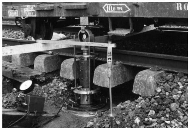
Figure 1. Plate Load Test during survey of railway subgrade
