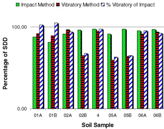
Figure 1. Comparison of Compaction Results for all Soils
