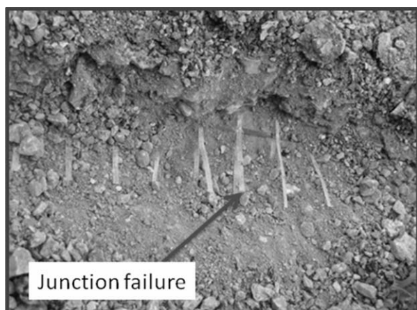
Figure 6. Separation of longitudinal and transverse ribs at junctions of Geogrid B at FM 1774
