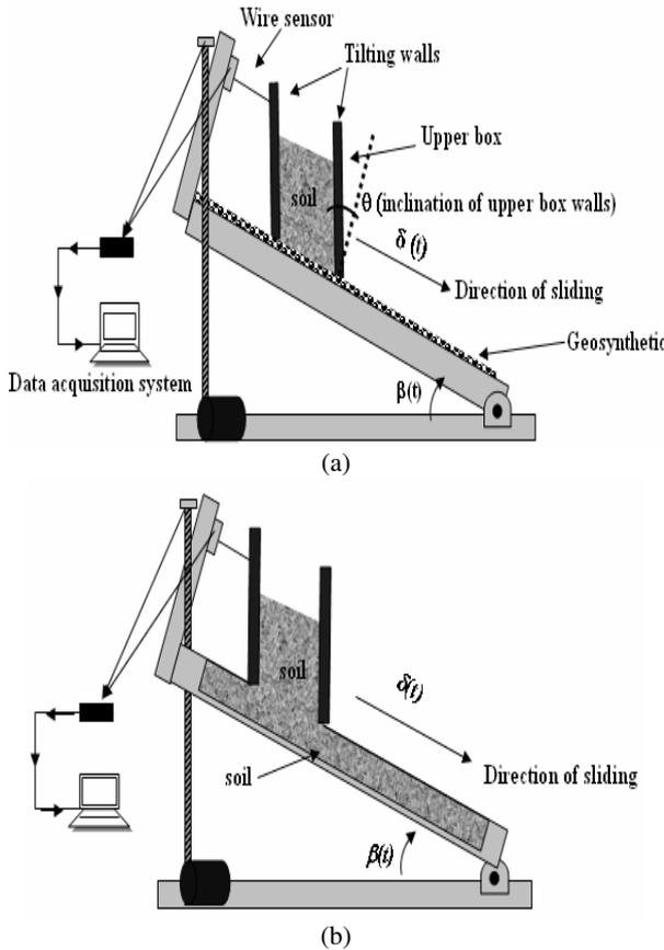
Figure 1. IPT for tests on soil-geosynthetic (a) and soil-soil (b) interfaces.
