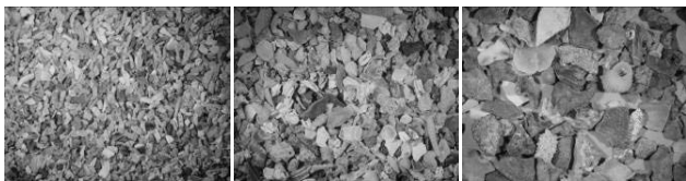
Figure 2 . Particle distribution for ranges: 0.15 to 0.25 mm; 0.25 to 0.5 mm and 0.5 to 1.0 mm.
