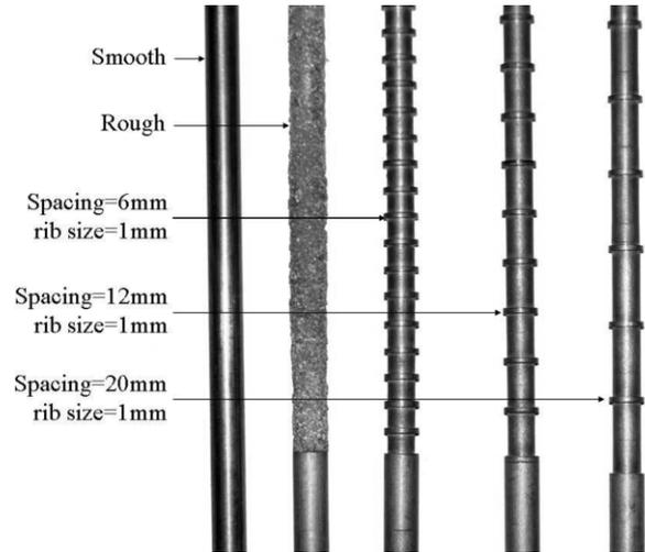
Figure 3. Types of anchors for the experimental study.
