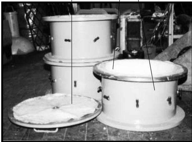
Figure 1. Triaxial test tank.
