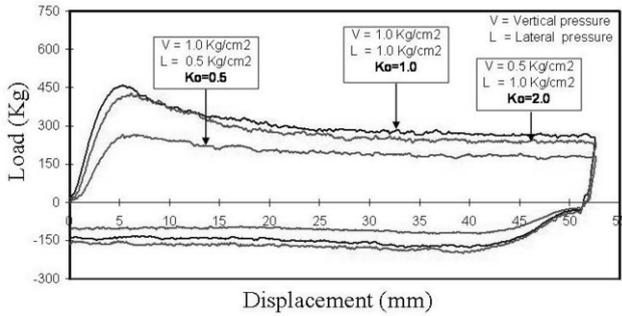
Figure 7. The effect of  $K_o$  on the pullout resistance.
