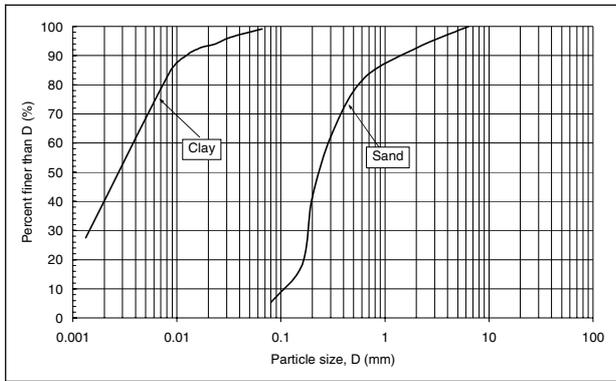
Figure 2. Particle size distributions of clay and sand used in model tests
