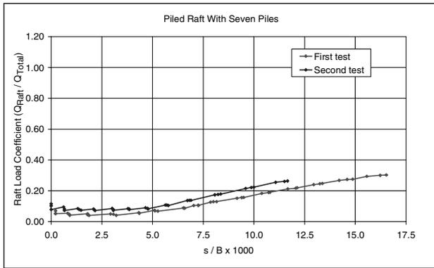
Figure 6. Raft load coefficient–settlement relationship of piled raft with seven piles
