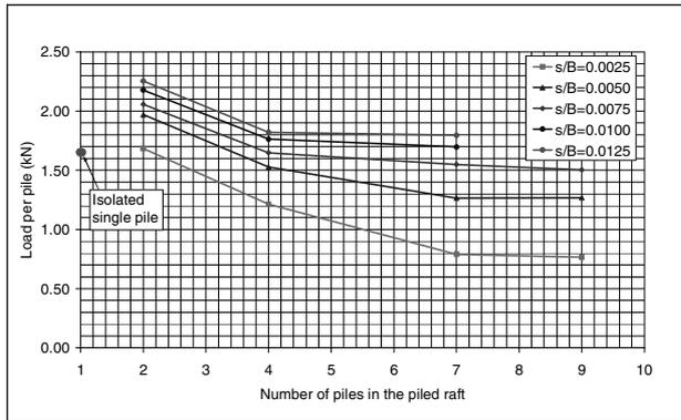
Figure 10. Effect of number of piles to the load carried by piles in piled rafts
