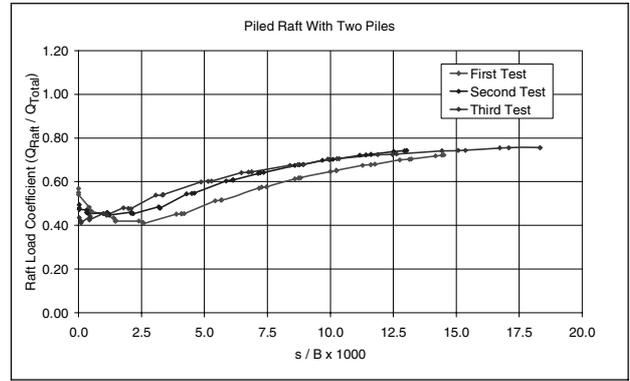
Figure 7. Raft load coefficient–settlement relationship of piled raft with two piles
