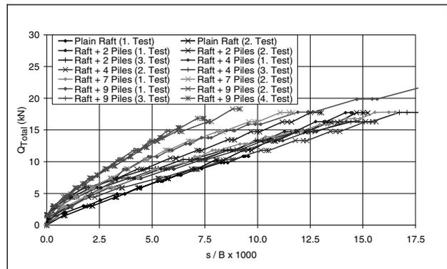
Figure 4. Load – settlement relationships of piled rafts and plain raft
