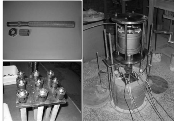
Figure 3. Model pile, piled raft and the loading system
