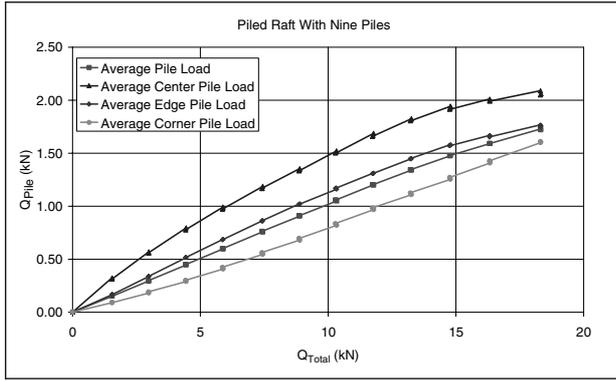
Figure 5. Average single pile loads for different locations of piles in the piled raft with nine piles
