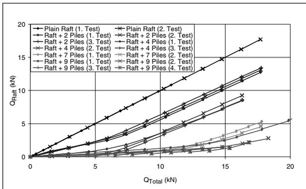
Figure 11. Load transferred by raft in different piled raft configurations
