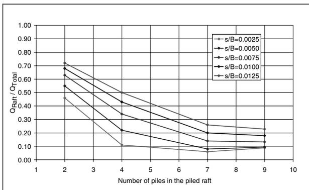
Figure 12. Effect of number of piles to the load carried by raft in piled rafts
