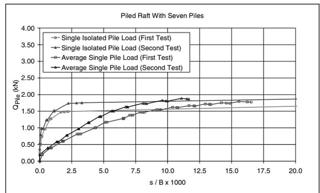
Figure 9. Load–settlement behavior of single pile in the piled raft with seven piles
