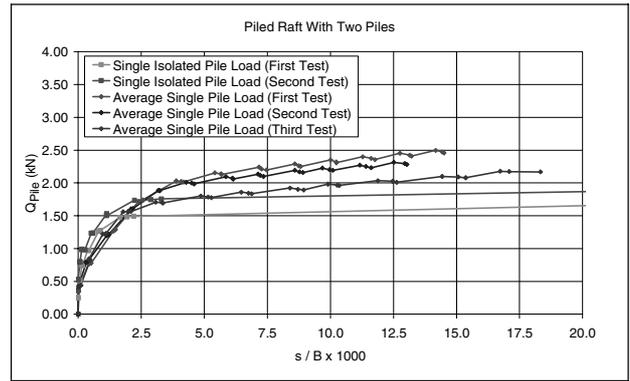
Figure 8. Load–settlement behavior of single pile in the piled raft with two piles
