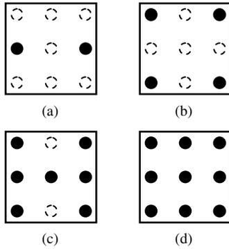
Figure 1. Model piled raft configurations: a) piled raft with two piles, b) piled raft with four piles, c) piled raft with seven piles, d) piled raft with nine piles
