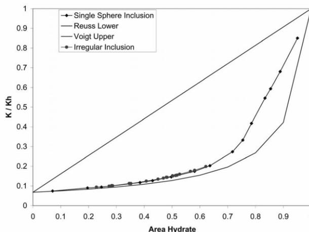
Figure 2. Normalized bulk modulus versus hydrate content within the sediment
