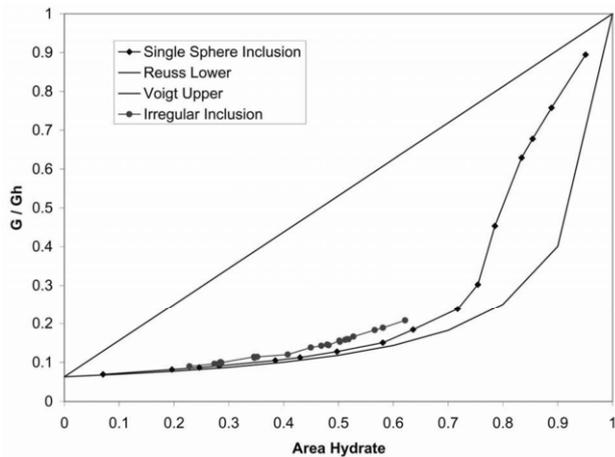
Figure 3. Normalized shear modulus versus hydrate content within the sediment
