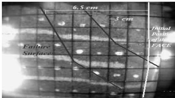
Figure 2. The first and second failure surfaces according to the target points and lines
