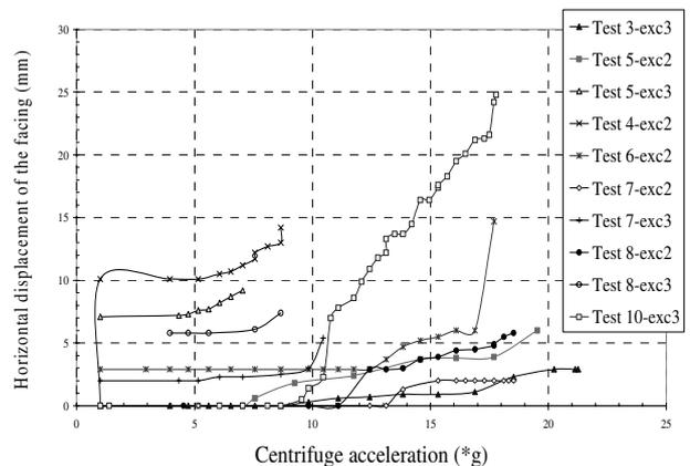
Figure 6. Horizontal displacements of the wall with increase of centrifuge acceleration
