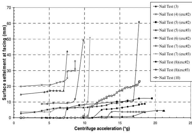
Figure 7. Settlement of top of the wall with increase of centrifuge acceleration
