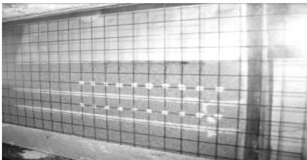
The horizontal displacement of the slope crest is measured by an LVDT and the logged data is stored in a computer attached to the arm of the centrifuge near the main vertical shaft. After the test, the data is analyzed. Different stages of excavation and acceleration are done in the same way until failure.
