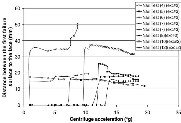
Figure 8. Variation of the first failure surface distance to the initial position of facing with acceleration
