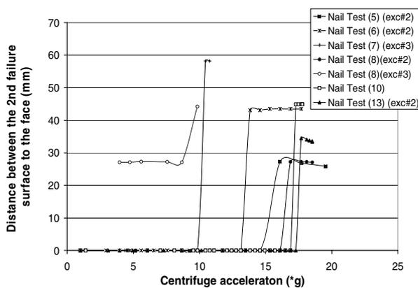
Figure 9. Variation of the second failure surface distance to the initial position of facing with acceleration
