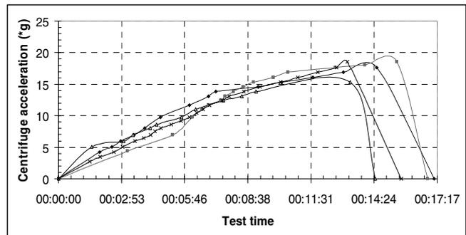
Figure 5. Centrifuge acceleration change during the tests
