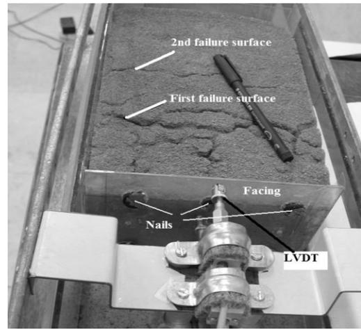
Figure 4. One model after failure – in which two failure surfaces can be seen
