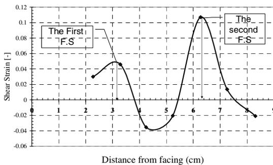
Figure 3. The shear strain change with distance on the side of the sample
