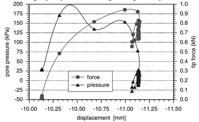
Figure 5. Relationship between pore pressure at the pile tip and penetration force as a function of pile displacement, Test 2 penetration velocity is 300 mm/s.
