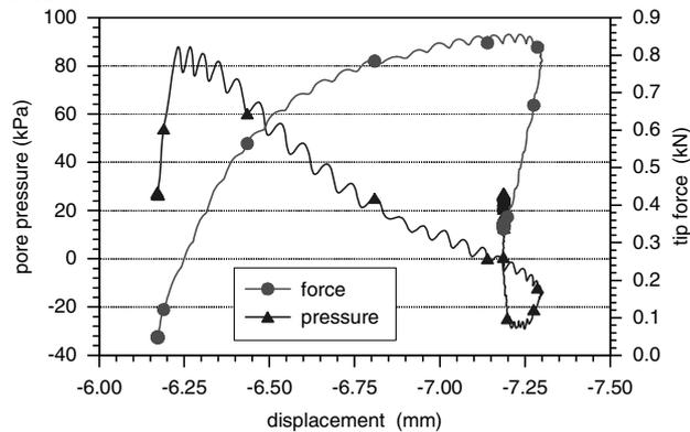
Figure 4. Relationship between pore pressure at the pile tip and penetration force as a function of pile displacement, Test 2 penetration velocity is 36 mm/s.
