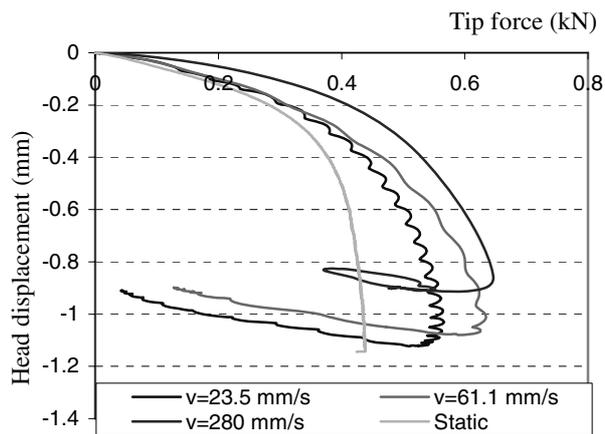
Figure 2. Force displacement diagram for different penetration velocities, Test 3.
