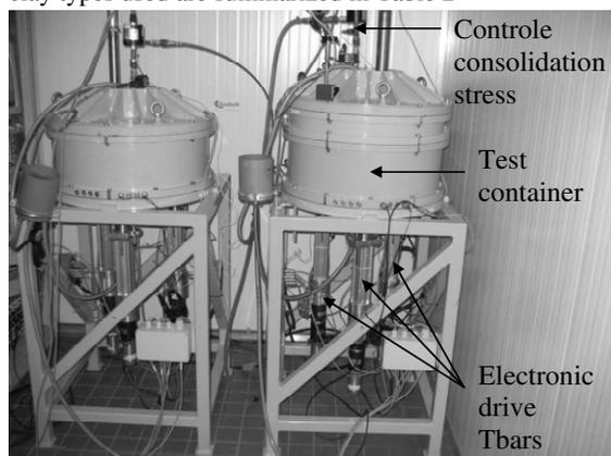
Figure 7. Test set-up of T-bar penetration tests showing test container filled with clay and electronic drive of the three T-bars
