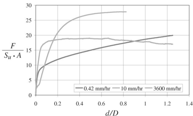
Figure 8. Diagram for different penetration rates of T-bar penetration in 'Oostvaardersplassen' clay, with force  $F$  normalized with the  $S_u$  and the area of the T-bar against the T-bar penetration  $d$  normalized with the diameter  $D$  of the T-bar.
