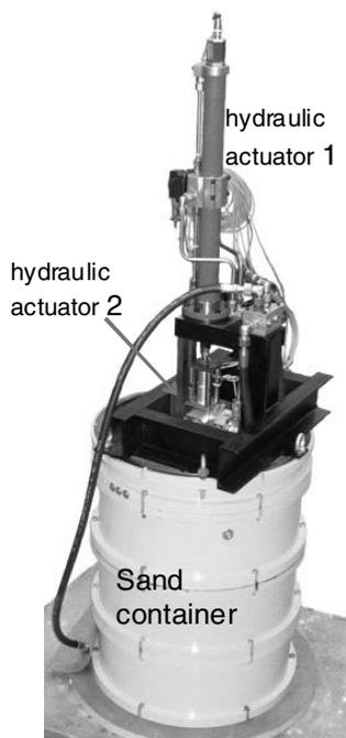
Figure 1. Test set-up for rapid pile tests in a geotechnical centrifuge.
