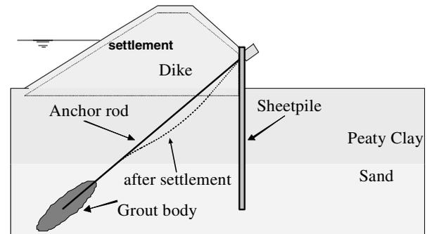
Figure 6. Sheet pile construction stabilized with grout anchor for dike-strengthening projects
