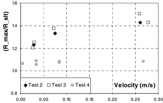
Figure 3. Comparison of rapid and static ultimate capacity for cases with viscous pore fluid (test 2 and 3) and with water (test 4)
