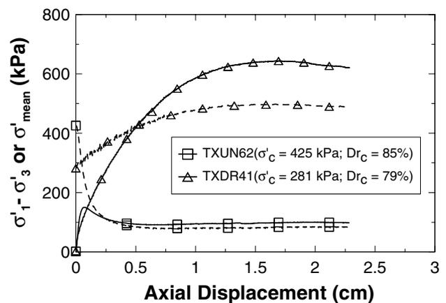
Figure 2. Example stress-displacement plots of TxC tests on air pluviated MR sand ( $\sigma_1 - \sigma_3 =$  solid line;  $\sigma'_{mean} =$  dashed line) -  $\sigma'_c$  is the consolidation mean stress.
