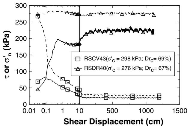
Figure 4. Example stress-displacement plots of RS tests on air pluviated MR sand ( $\tau$  = solid line;  $\sigma'_n$  = dashed line) -  $\sigma'_c$  is the consolidation normal stress.
