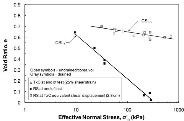
Figure 5.  $CSL_o$  and  $CSL_c$  from shears and TxC tests.
