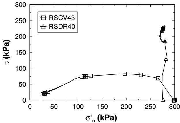
Figure 3. Example stress paths of RS tests on air pluviated MR sand
