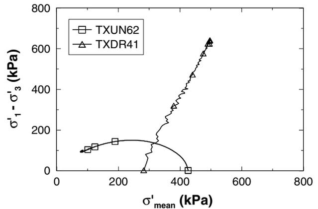
Figure 1. Example stress paths of TxC tests on air pluviated MR sand
