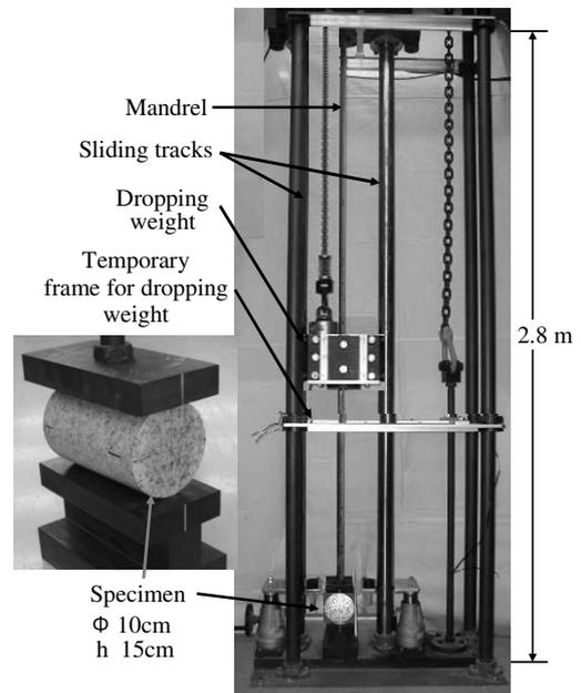
Figure 1. Impact testing machine.
