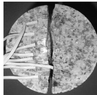
Figure 7. Test specimen after impact splitting tests.
