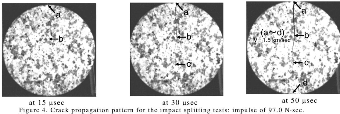
Figure 4. Crack propagation pattern for the impact splitting tests: impulse of 97.0 N·sec.
