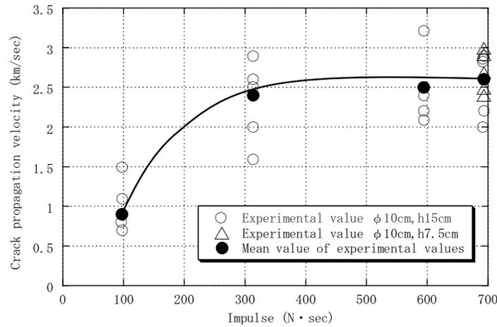
Figure 5. Relationship between the impulse and the crack propagation velocity.
