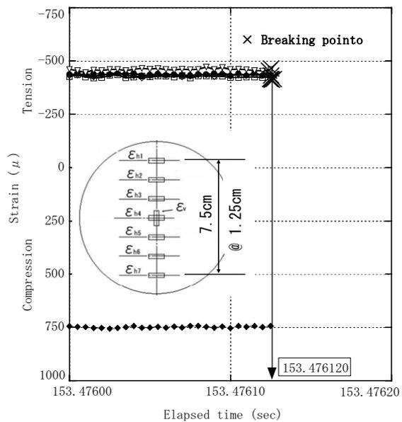
Figure 3. Measuring results for static strain: loading speed of 70 kN/min.
