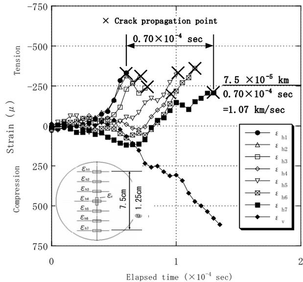
Figure 6. Measuring results of dynamic strain: impulse of 97.0 N·sec.
