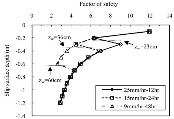
Figure 4.2: Variation of factor of safety along slip surface. (Lee *et al.*, 2009)
