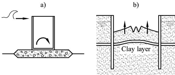
Figure 2.3: Two failure scenarios which cannot be properly handled by a  $(c', \phi')$  reduction method: (a) Overturning failure of a caisson against external horizontal loading. (b) Bottom instability of an excavation due to non compensated water pressures.
