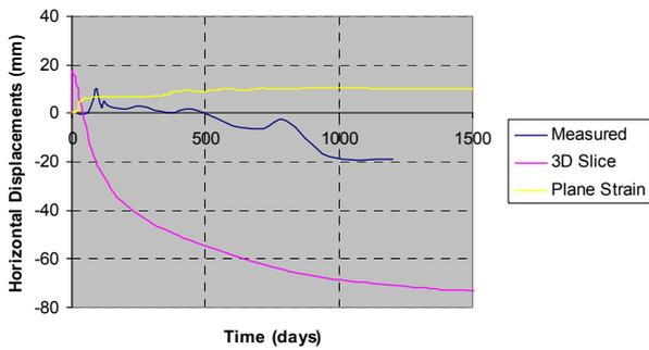
Figure 4.7: Comparison of horizontal deformations (Montgomery and Karstunen, 2009).
