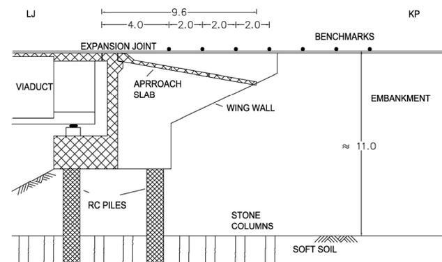
Figure 3.12: Longitudinal section of the embankment at the viaduct.
