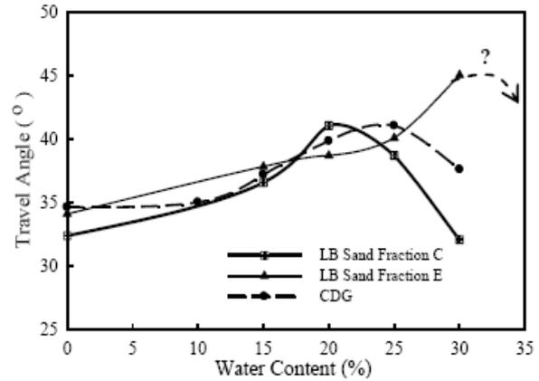
Figure 2.12: Effect of water content on flow mobility (Zhou *et al.*, 2009)
