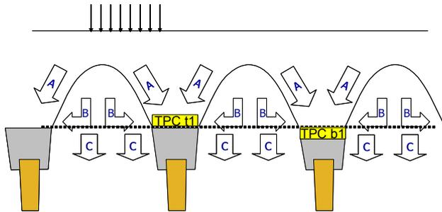
Figure 3.1: Load distribution into load parts A, B and C. Locations of Total Load Pressure Cells (TPC's) in the Kyoto Road field test (Van Eekelen *et al.*, 2009).
