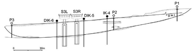
Figure 3.10: Cross-section down the middle of the sliding mass with pier S3. (Nossan *et al.*, 2009)
