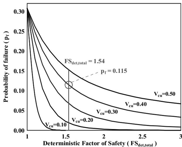
Figure 7.6: Probability of failure as a function of the deterministic factor of safety ( $FS_{det}$ ) and the variability index of  $c_u$  ( $V_{c_u}$ ) for slopes in cohesive soil under undrained conditions. (Kavvasdas *et al.*, 2009)
