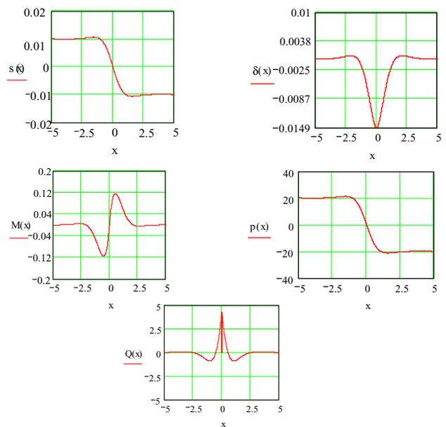
Figure 2.7: Displacements  $s(x)$ , inclinations  $\delta(x)$ , bending moments  $M(x)$ , shear forces  $Q(x)$ , soil reactions  $p(x)$  (tons and meters) (Barvashov *et al.*, 2009).
