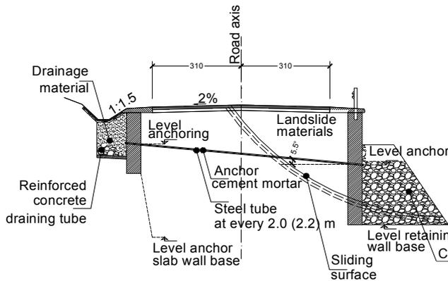
Figure 7.1: Anchored walls- plates. (Hamova *et al.*, 2009)
