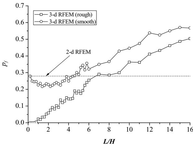
Figure 7.5: Probability of failure versus slope depths ( $\Theta_{c_u} = 2.0$ ,  $v_{c_u} = 0.5$ ) (Griffiths *et al.*, 2009).
