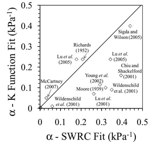
Figure 6.5: Comparison between  $\alpha$  parameters for different soils obtained from fitting the van Genuchten (1980) model to the k-function data and to the SWRC data. (McCartney and Parks, 2009)
