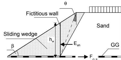
Figure 3.3: Sliding soil wedge to determine the spreading force (Fahmy *et al.*, 2009)
