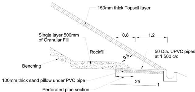
Figure 3.6: Typical design of filter layer and contour drain channel. (Mickovski and Smith, 2009)
