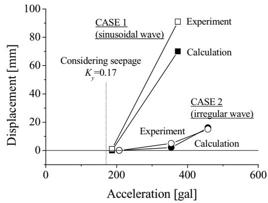
Figure 5.1: Residual displacement of calculation and experiment (Matsumaru *et al.*, 2009).
