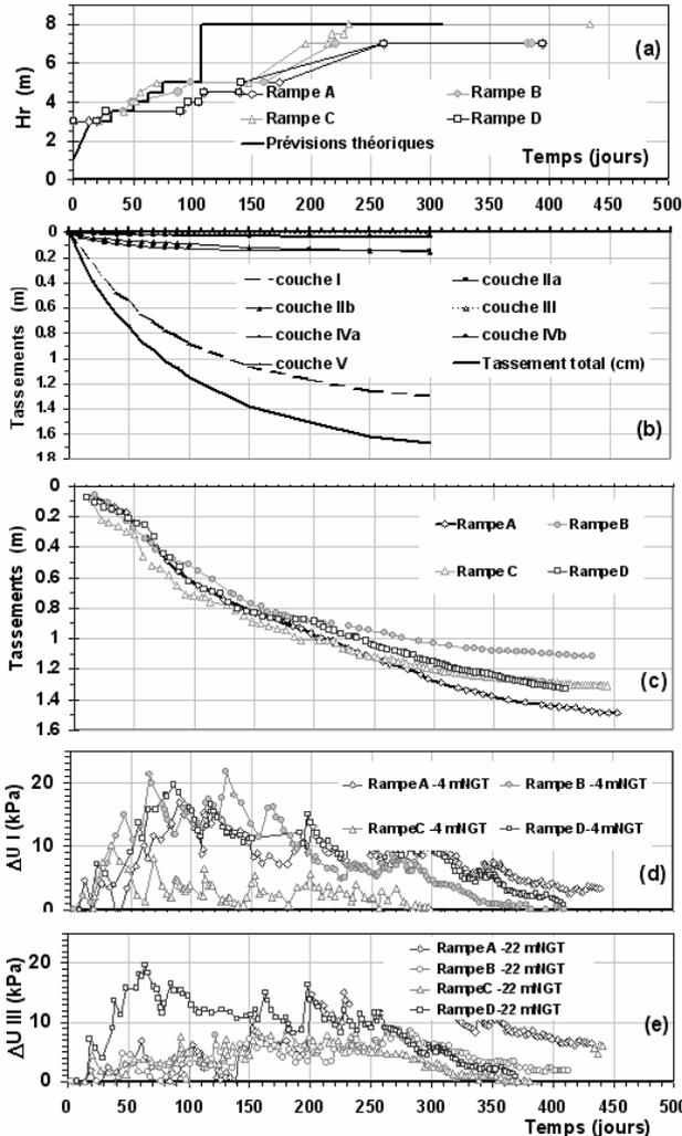
Figure 6.1: Synthesis of the different estimations and measurements after preloading. (Zaghouani *et al.*, 2009)
