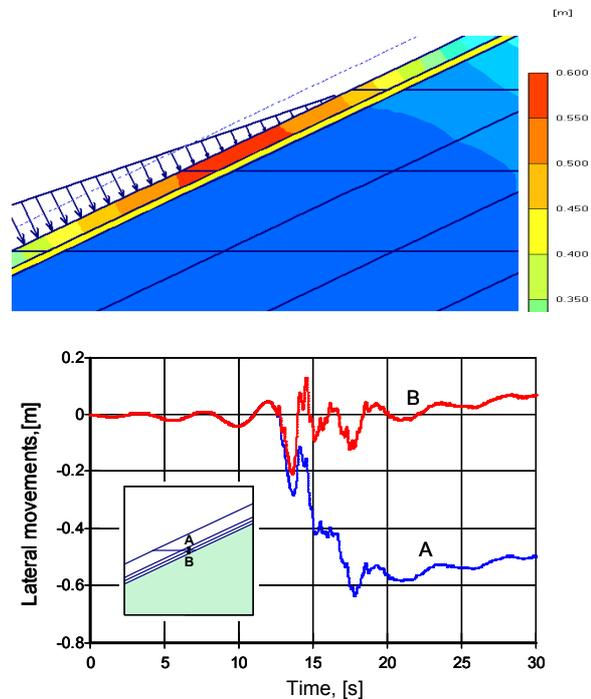
Figure 5.5: (a) Close up of the largest deformation from the time history at Hella. (b) History of the lateral movement of two points A and B on each side of the geomembrane during the earthquake loading. (Erlingsson and Hauksson, 2009)
