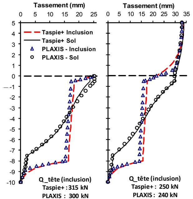
Figure 2.6: Settlement profiles calculated for two configurations: paving (left) and embankment (right). (Cuira and Simon, 2009).
