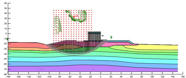
Figure 2.2 LE failure analysis (Morgenstern-Price method, circular failure surface) of caisson under static horizontal wave loading and selfweight.
