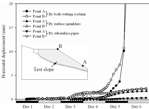
Figure 4.1: Comparison of wetting induced horizontal displacements by different infiltration schemes (Zhou *et al.*, 2009)
