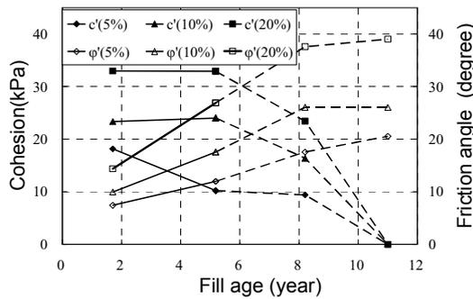
Figure 3.9: Relationships of shear strength parameters to the fill age of MSW (Chen *et al.*, 2009).
