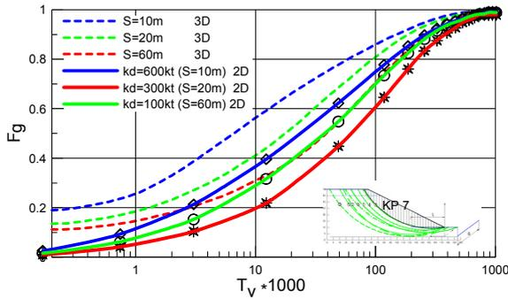
Figure 4.6: The gain in the factor of safety  $F_g$  versus the time factor  $T_v$  for slip surface 7 (critical slip surface)  $L=50m$ ,  $S=10, 20, 60m$ . (Gjetvaj *et al.*, 2009)
