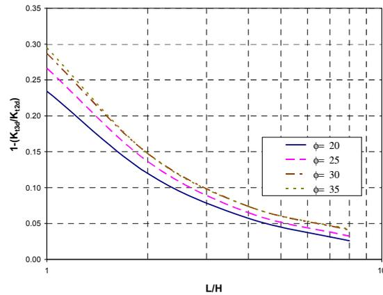
Figure 2.9: Required reinforcement strength ( $\beta = 80$ ) (Askari *et al.*, 2009).
