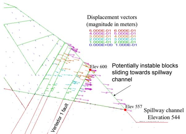
Figure 7.4: Detail of displacements at slope's toe for maximum credible earthquake (Tr10000). (Méndez *et al.*, 2009)
