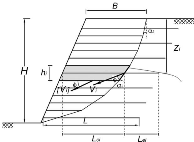
Figure 2.8: Transitional multi-block mechanism (Askari *et al.*, 2009).
