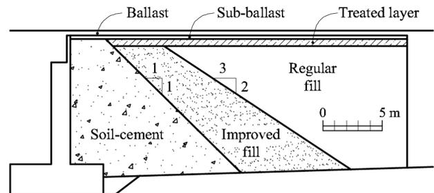
Figure 3.11: Example of transitional wedge to a railway bridge abutment.
