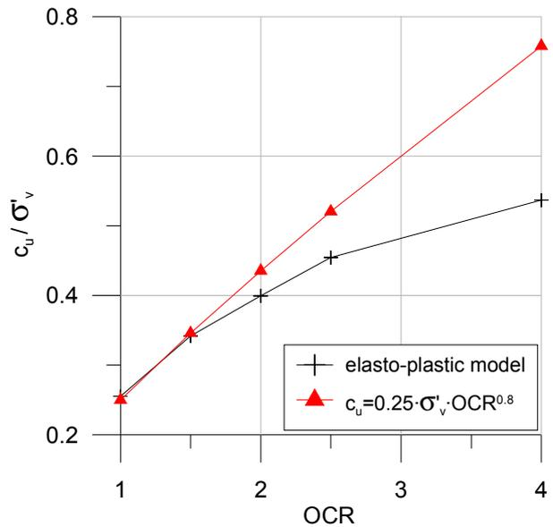
Figure 2.4: Simulation of undrained FE simple shear.
