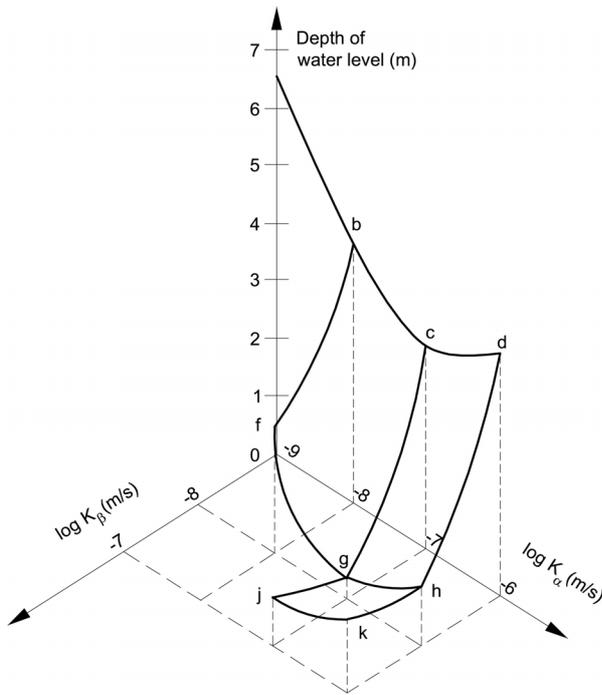
Figure 4.3: Computed depth of water level at piezometer P5699 for the time  $t = 350$  days after the beginning of the prediction exercise (October 1st, 1992). Depth of sensor: 2.80 m (Alonso *et al.*, 2003).
