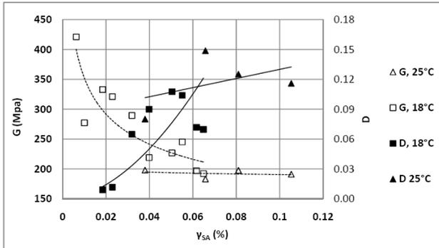
Figure 6.3: Effects of temperature on  $G$  and  $D$ , M.A.S.=12.7 mm,  $b$ =5.5% and  $\sigma_3$ =400 kPa (Jafarzadeh and Yousefpour, 2009).
