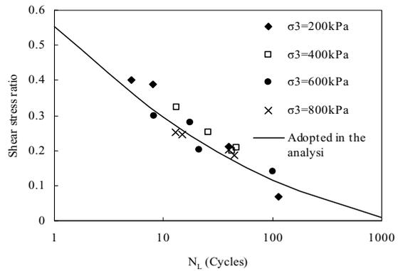
Figure 5.2: Number of cycles to cause liquefaction of filter layer. (Han-long and Kank, 2009)
