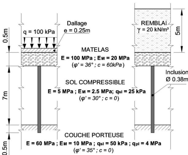
Figure 2.5: Example of reinforcement by means of stiff inclusions (Cuira and Simon, 2009).
