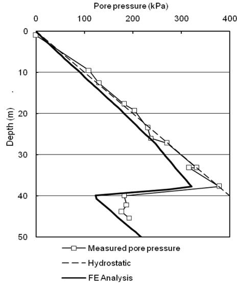
Figure 4.5: Measured and predicted by FEM initial pore-pressure profile (Bardanis *et al.*, 2009).
