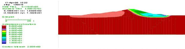
Figure 5.6: x-displacement contours within the body of the dam section indicating a base type failure due to presence of liquefiable layer. (Sivakumar and Srivastava, 2009)
