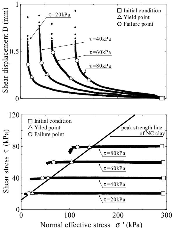
Figure 2.11: Stress controlled ring shear test for virgin type landslide (Ohtsuka and Isobe, 2009).
