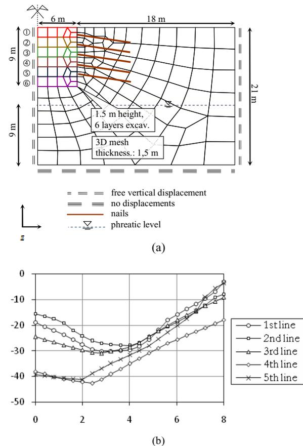
Figure 2.10: (a) Vertical excavation with soil nailing. (b) Axial forces in the reinforcements at the end of excavation (Farias and Durand, 2009).
