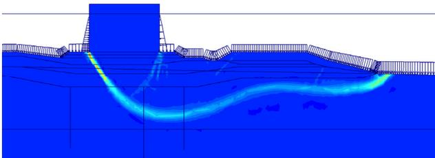
Figure 2.1 Failure surface developed in a  $(c', \phi')$  reduction method.
