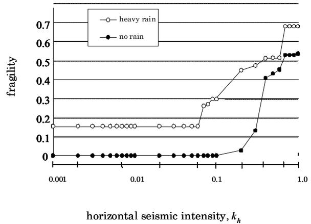
Figure 7.3: Fragility intensity with respect to the seismic intensity. (Sumi *et al.*, 2009)
