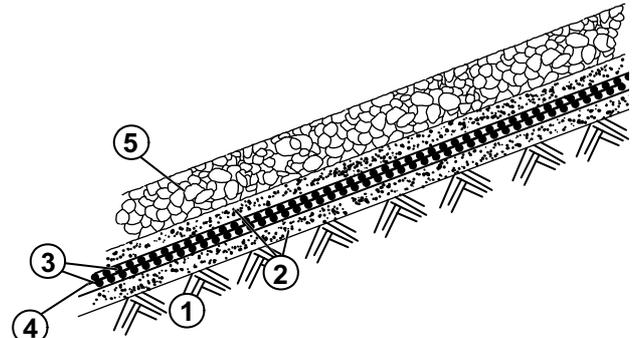
Figure 5.4: Details of the geomembrane facing. 1, Earthfill; 2, crushed gravel; 3, non-woven geotextile; 4, geomembrane; 5, rockfill (after Girard *et al.*, 1990).
