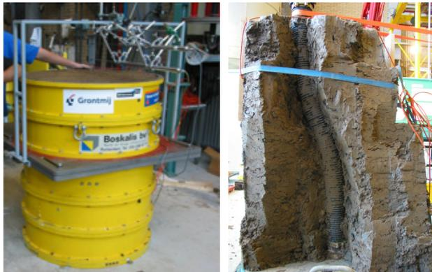
Figure 3.2: Large-scale Direct Shear test on nails in clay (Lengkeek and Bruijn, 2009).
