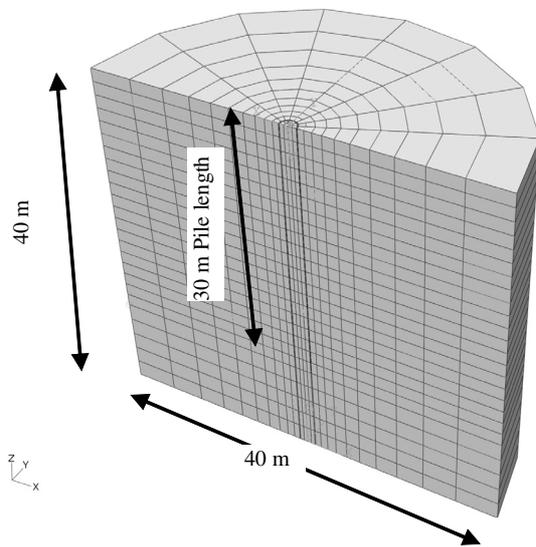
Figure 2. Finite Element Mesh for 2 m diameter and 30 m length steel pipe pile.
