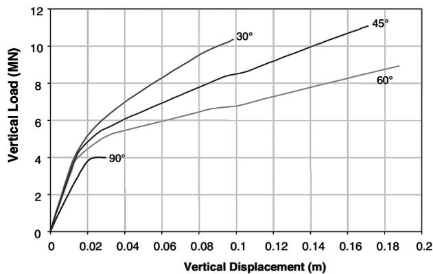
Figure 4. Vertical load versus vertical displacement curves at pile head for different inclination load angles.
