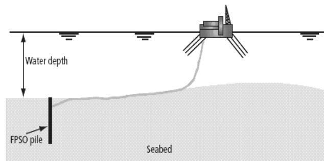
Figure 1. Schematic diagram of an FPSO and Anchoring System (after Bhattacharya 2007).
