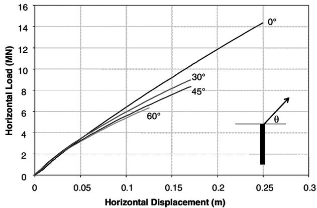
Figure 3. Horizontal load versus horizontal displacement curves at the pile head for different inclination load angles.
