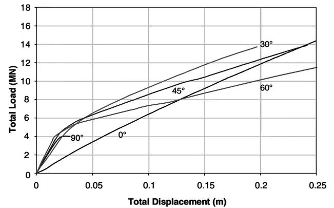
Figure 5. Total load versus total displacement curves at pile head for different inclination load angles.
