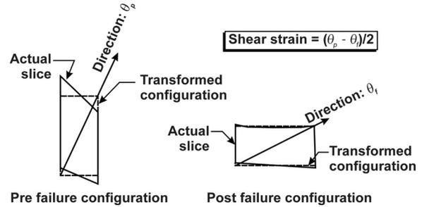
Figure 2. Shear strain estimation
