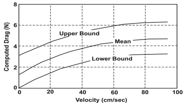
Figure 3. Viscous drag force - velocity relationships (after de Alba and Ballesterro 2006)
