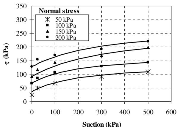
Figure 6. Shear strength envelopes in the space (s,τ) adjusted according to the hyperbolic function used by Gens (1993).
