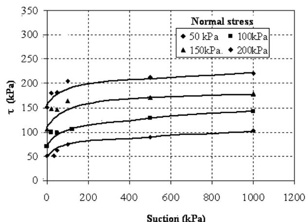
Figure 7. Shear strength envelopes in the space (s,τ) adjusted according to the hyperbolic function used by Gens (1993) – mature residual soil of granite (Lafayette, 2006).
