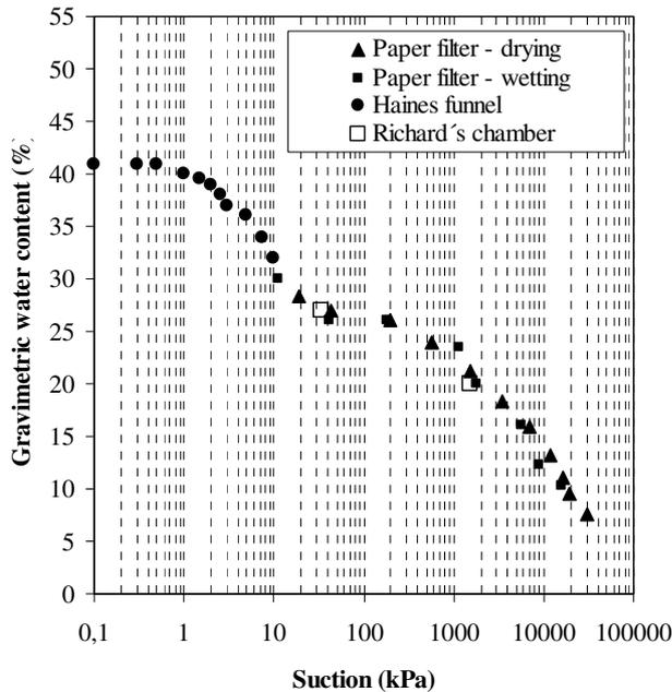
Figure 4. Soil-water characteristic curve obtained through the paper filter, Haines Funnel and Richard's chamber methods.
