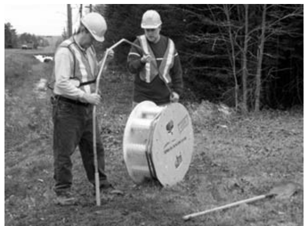
Photo-2 MEMS based multi points Tilt sensor < http://www.measurandgeotechnical.com >
