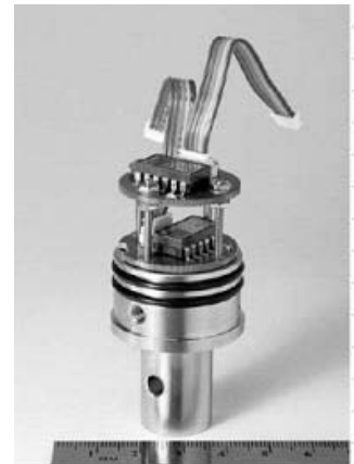
Photo-1 Biaxial Tilt Sensor (Two sets of MEMS Tilt sensor in a perpendicular position each other) Geokon biaxial sensor
