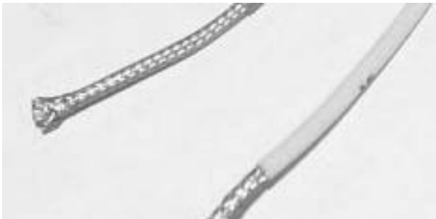
Figure 3.9. TDR cables: 0.59 mm diameter 75 \Omega (left), 1.02 mm diameter 50 \Omega (right) (McAlister & Pierce 2001).
