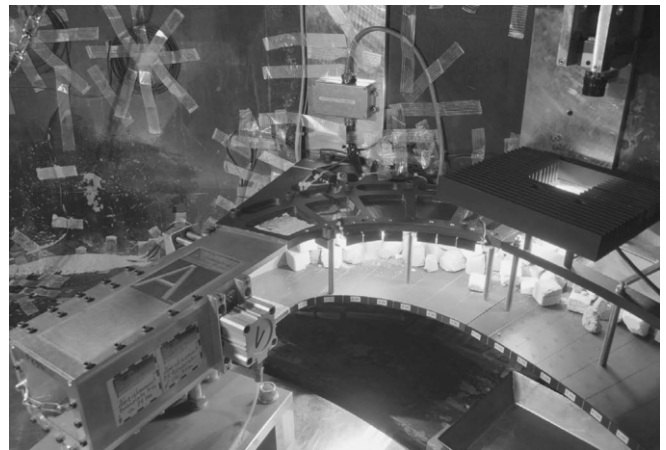
Figure 3.33. Run-out chute showing fragmented boulders after a rock avalanche event (Imre 2008).
