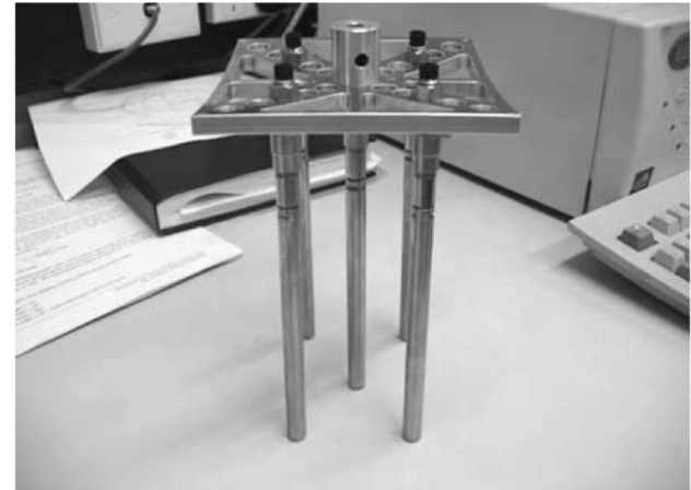
Figure 3.15. Installation of piles; a) influence of methods, in-flight or on ground, on pile normalized lateral pressure p\gamma/d with \gamma unit weight and d pile diameter (Dyson & Randolph 2001); b) pile group (Gaudin & Lehane 2006).
