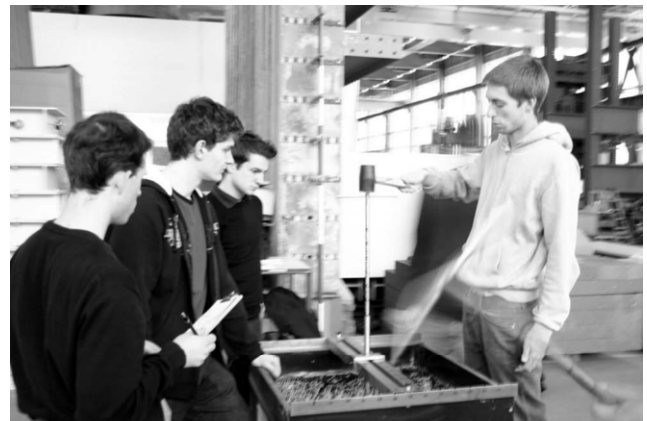
Figure 4. Students driving the sampler into the model.
