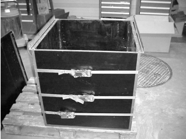
Figure 1. Wooden Box containing the soil sample. A guiding bar is attached left and right with the North – South (Fig. 2) coordinates of the model.
