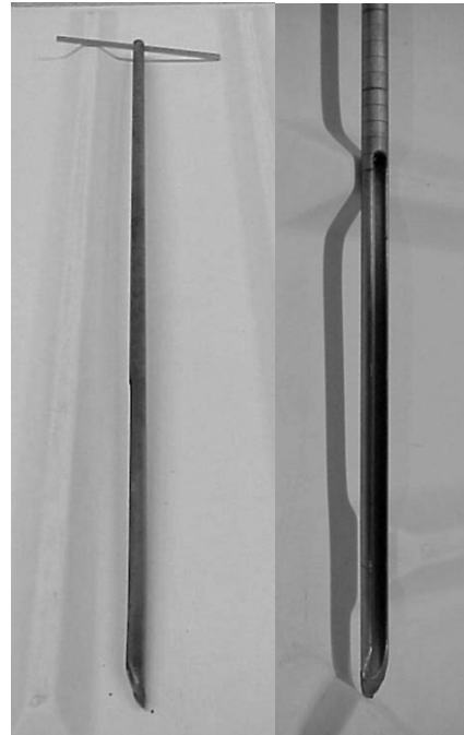
Figure 3. Slotted sampler with marked heights on the shaft.
