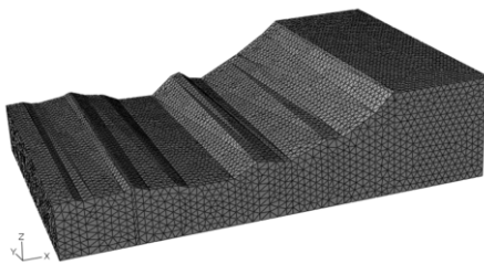
Figure 3 . FE-mesh on the wire-frame model from Figure 2
