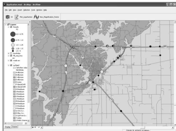
Figure 4. S4 Liquefaction Potential Results for 224 Year Mean Return Time Ground Motion.
