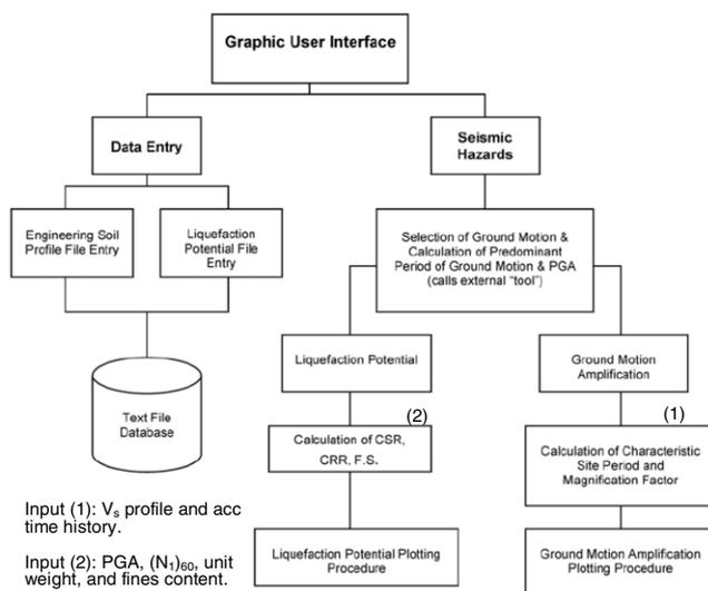
Figure 1. System architecture for prototype application (S4).
