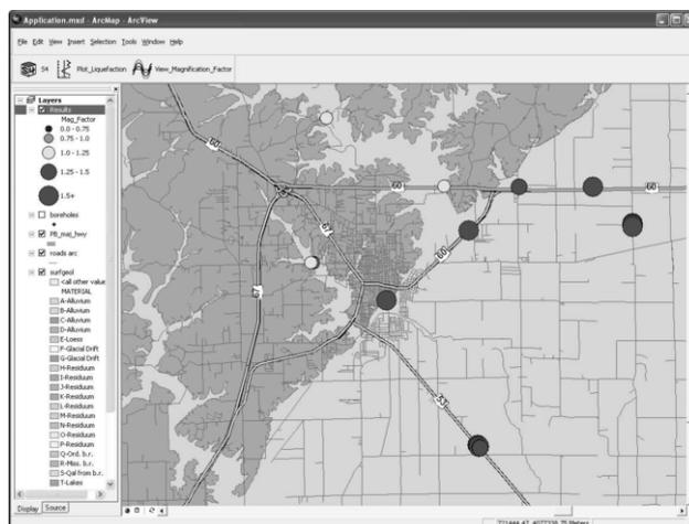
Figure 3. S4 Ground Motion Magnification Factor Results for 224 Year Mean Return Period Ground Motion.
