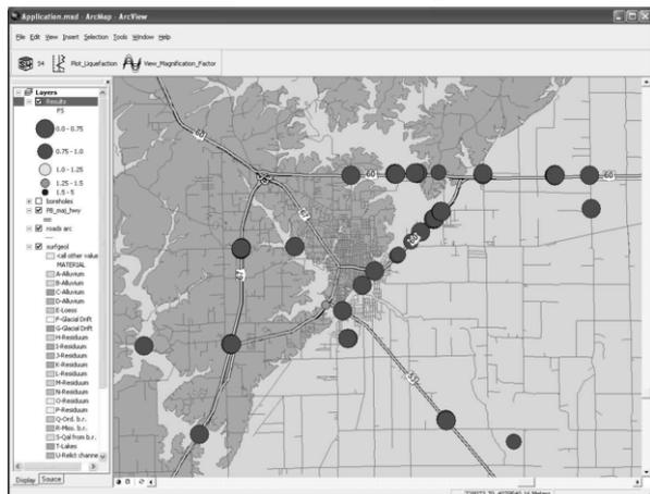
Figure 6. S4 Liquefaction Potential Results for 2475 Year Mean Return Period Ground Motion
