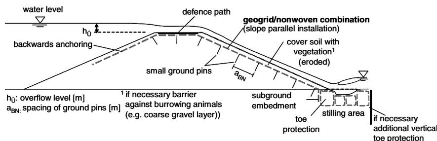
Figure 4. Overflow defense Method II, embankments with geogrid-geocomposite system and soil nails (Haselsteiner et al. 2008)
