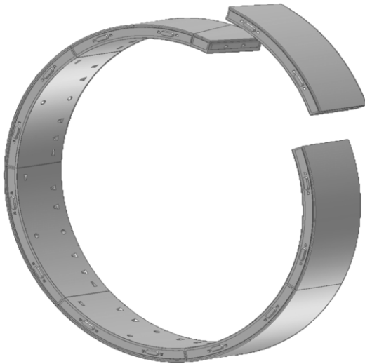
Figure 1: Realistic simulation of tunnel lining
