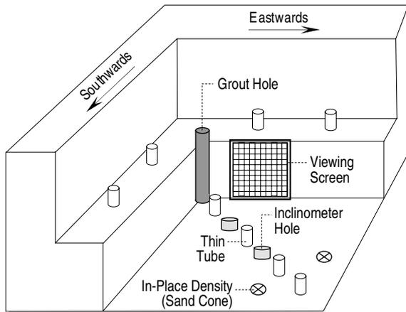
Figure 1. Illustration of excavated site & sampling locations.
