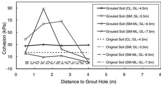
Figure 6. Cohesions of grouted soils.
