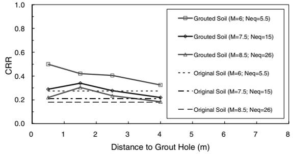
Figure 8. Liquefaction resistance of grouted sand at GL:-5.5m.
