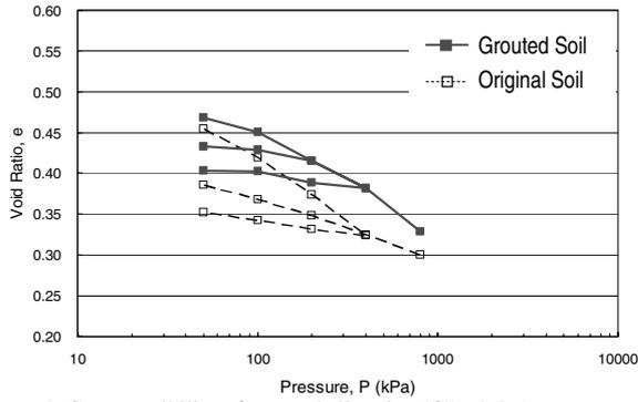
Figure 4. Compressibility of grouted silty clay (GL:-4.5m).
