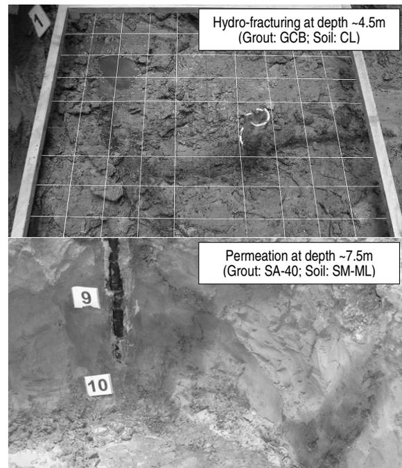
Figure 3. Observed mechanisms of grout injection.
