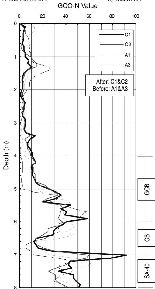
Figure 2. Improved depth intervals of penetration resistance.
