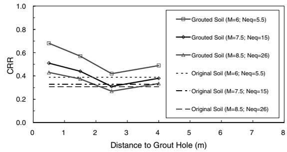
Figure 7. Liquefaction resistance of grouted sand at GL:-5.5m.
