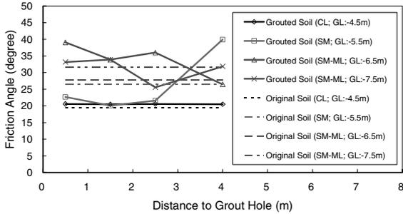
Figure 5. Friction angles of grouted soils.
