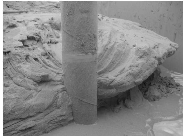
Figure 6 Detail of the cemented sand body close to the extraction point shows that the cemented patterns are clearly related to the flow paths through the sand body.
