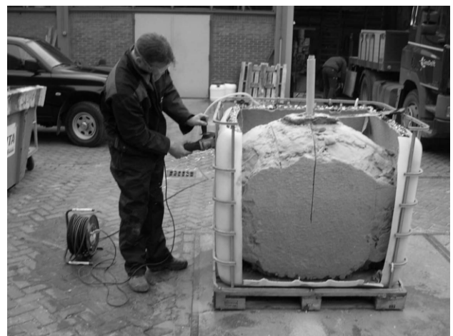
Figure 3 The spherically shaped cemented sand body.
