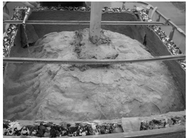
Figure 2 The surface of the cemented sand body of the second cubic meter test. Ridges with high \text{CaCO}_3 content are visible in a regular pattern on the left.
