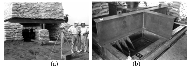
Fig. 4. Load Test Arrangement on Group of Granular Piles (a) Dead Load Kentledge (b) Close-up View of Test Plate and Dial Gauge
