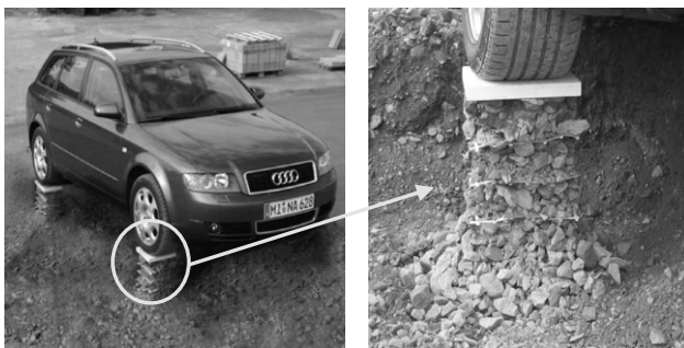
Figure 3. Lateral restraint of aggregate using high modulus laid and welded geogrids
