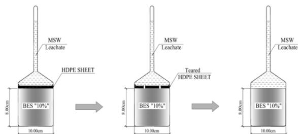
Figure 2: Falling Head Test on the Composite Liner
