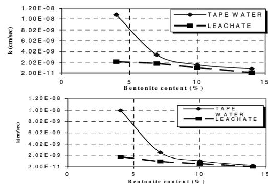
Figure 4: Bentonite content vs. the coefficient of permeability at different vertical stress
