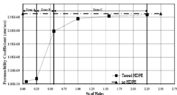
Figure 6: Percentages of Holes in the HDPE vs. Permeability.
