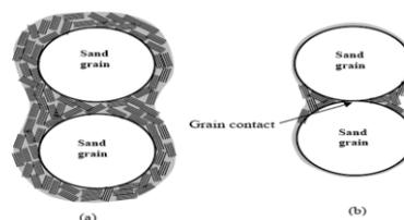
Figure 1: Two possible states of sand grains in a deflocculated clay system: (a) clay particles 'coating' sand grains and (b) clay particles 'welding' sand grains.
