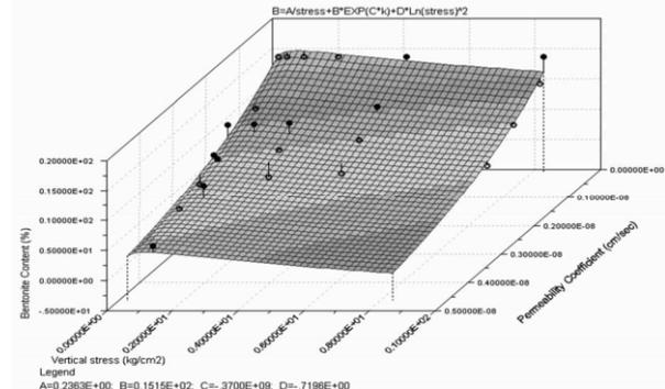
Figure 5: Relation between Bentonite Content, the Vertical Stress and the Permeability Coefficient.
