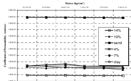
Figure 3: Vertical stress vs. coefficient of permeability (tape water).
