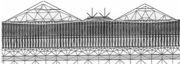
Fig. 6: Deformation prediction at runway corridor by FE-analysis.
