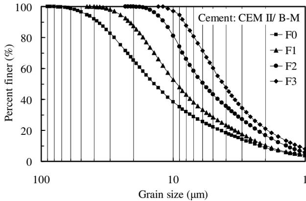
Figure 1. Grain size distributions of cements.
