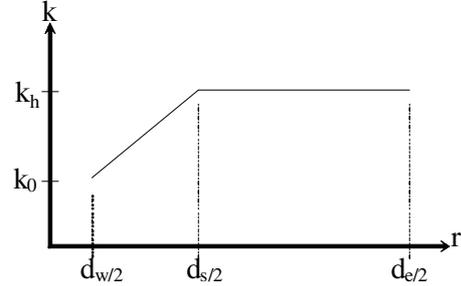
Figure 3. Linear variation of permeability in the smear zone
