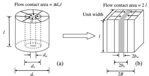
Figure 4. Unit cell analysis: (a) axisymmetric condition, (b) equivalent plane strain condition (after Indraratna et al., 2005)
