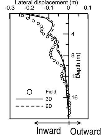
Figure 10. Lateral displacements at embankment toe at 168<sup>th</sup> day
