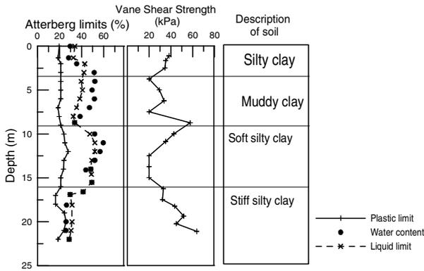
Figure 5. Soil properties and profile at Tianjin port (adopted from Rujikiatkamjorn et al. 2008)
