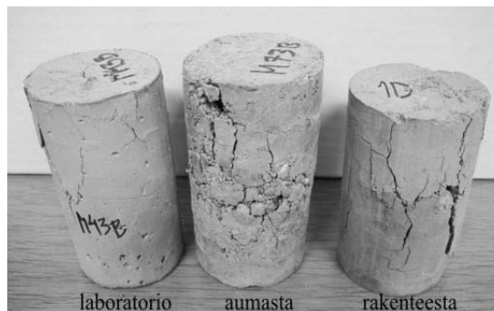
Figure 2. Laboratory and field specimens after unconfined compression test and drying in the oven. From the left: laboratory specimen S, heap specimen K1 and structure specimen K2.
