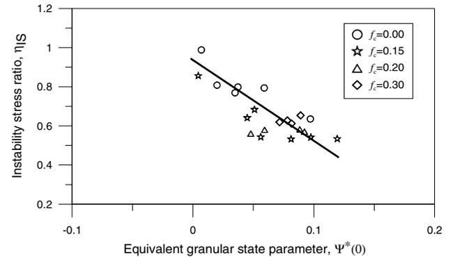
Figure 4. The relation between equivalent granular state parameter,  $\psi^*(0)$  and instability stress ratio,  $\eta_{IS}$  for sand with fines,  $f_c \leq TFC$ .
