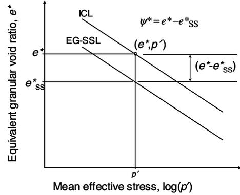
Figure 3. Definition of equivalent granular state parameter,  $\psi^*$
