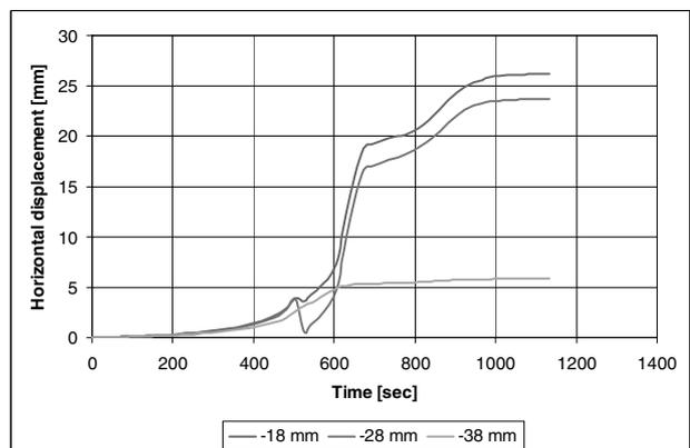
Figure 7. Horizontal deformation at 3 different ground levels in centrifuge test
