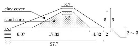
Figure 2. Test set-up, cross section dimensions in [m]
