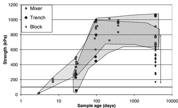
Figure 3. UCS result with time for CB samples
