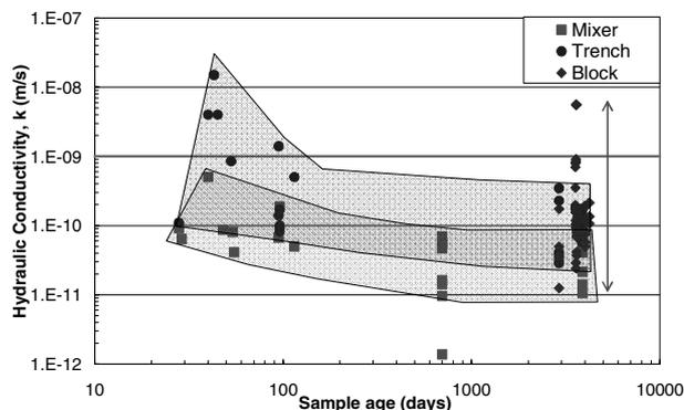
Figure 2. Hydraulic conductivity result with time for CB samples
