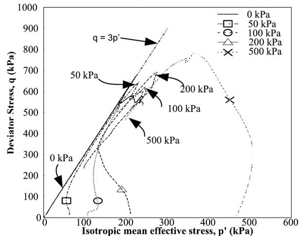
Figure 5. Stress path of triaxial test on 11 year old CB 'block' sample
