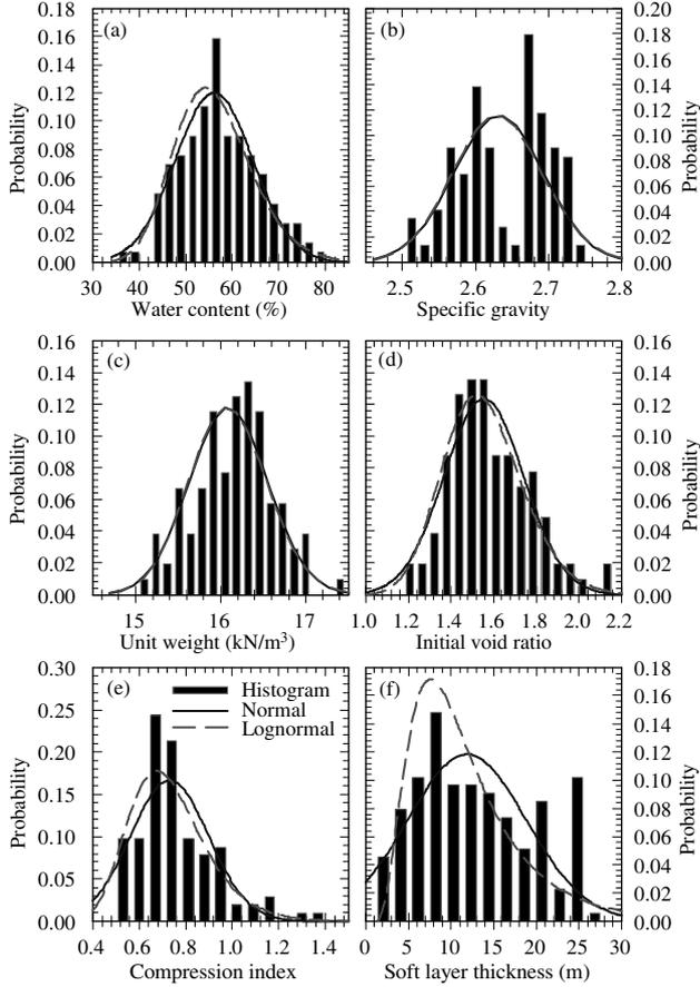
Figure 3. Probability density functions for the soil parameters.
