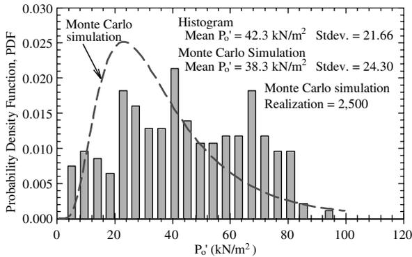
Figure 5. Distributions of the effective overburden pressures.
