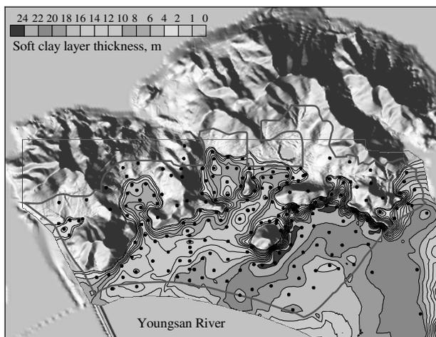
Figure 2. Contour map of H and locations of borings and Dutch-cones.
