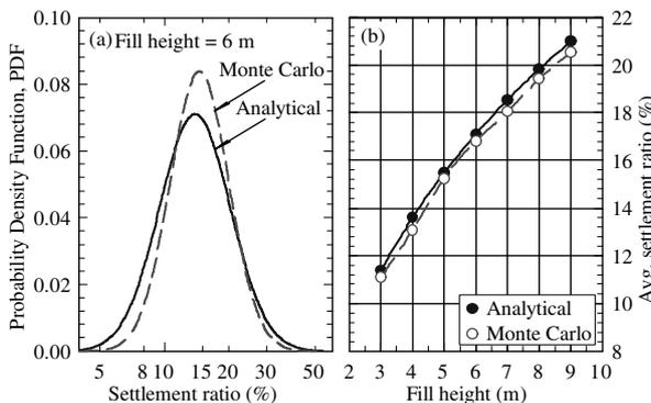
Figure 6. (a) Settlement ratio distributions for fill height of 6 m and (b) average settlement ratios for different fill heights.
