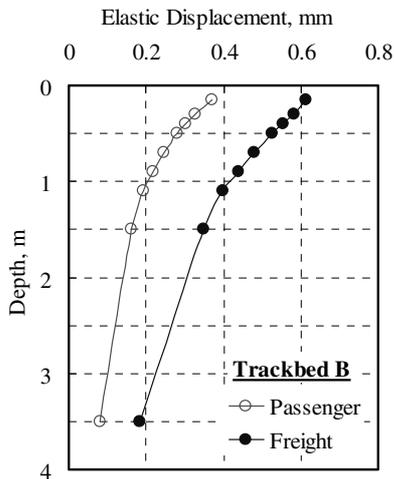
Figure 10. Vertical displacements of trackbed B.
