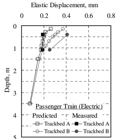
Figure 12. Comparison of displacements under passenger train.
