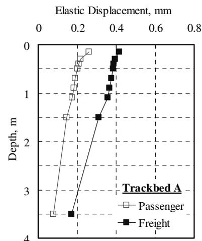
Figure 9. Vertical displacements of trackbed A.
