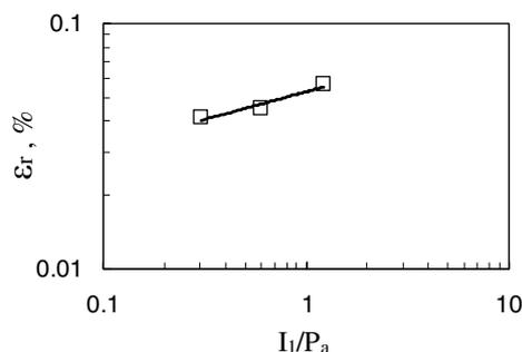
Figure 5. Relationship of  $\epsilon_r$  and  $I_1/P_a$  for weathered soil.
