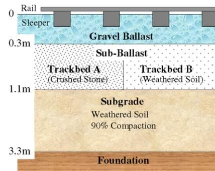
Figure 8. Layer system of trackbed A and B.
