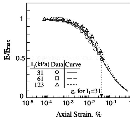
Figure 4. Plot of  $E/E_{max}$  vs.  $\epsilon$  for weathered soil.
