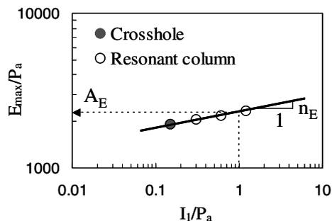
Figure 3.  $A_E$  and  $n_E$  of weathered soil.
