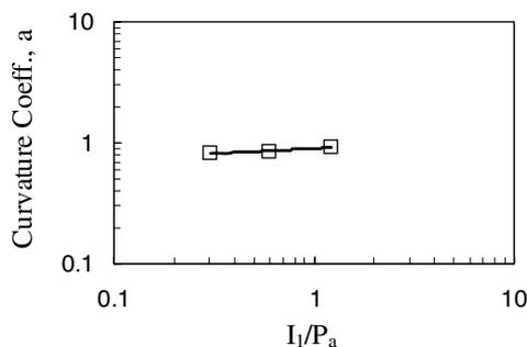
Figure 6. Relationship of  $a$  and  $I_1/P_a$  for weathered soil.
