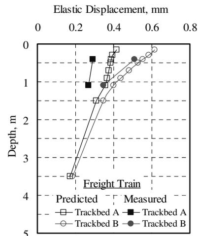
Figure 13. Comparison of displacements under freight train.
