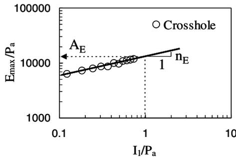
Figure 7.  $A_E$  and  $n_E$  of crushed rock-soil mixture.
