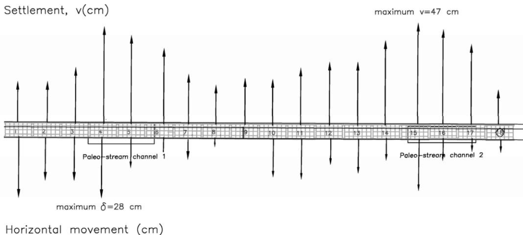
Figure 6.- Plan view with the maximum movements at the Bajo de la Cabezueta quay
