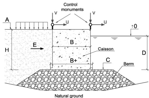
Figure 1.- Cross-section of a typical quay wall
