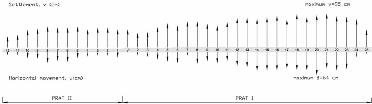
Figure 12.- Plan view with the maximum movements at the Prat quay
