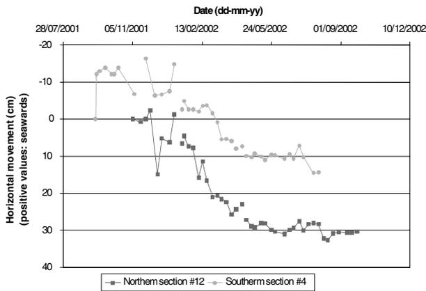
Figure 8.- Horizontal displacements at León y Castillo quay wall
