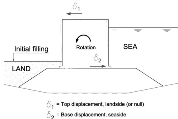
Figure 15.- Initial horizontal displacement
