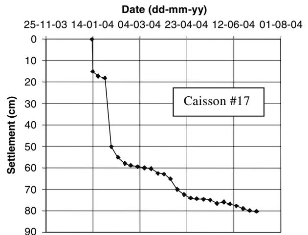
Figure 13.- Settlements at the Muelle n° 9 quay wall in Málaga
