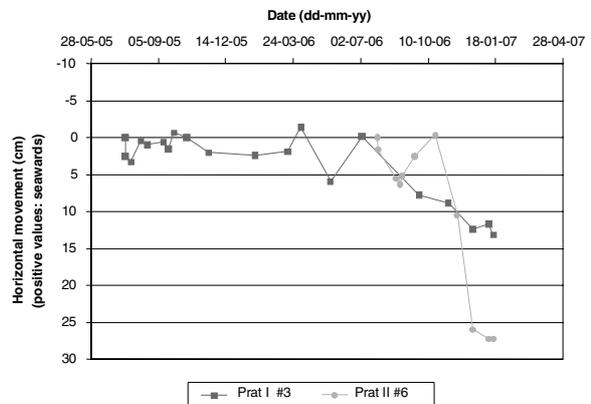
Figure 11.- Horizontal displacements at Prat quay wall
