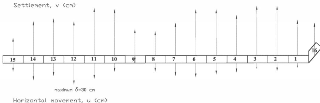
Figure 9.- Plan view with the maximum movements at the León y Castillo quay
