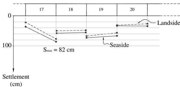
Figure 14.- Plan view of the Muelle nº 9 quay with the maximum settlement recorded
