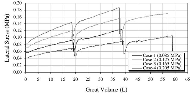
Figure 8. Lateral soil stress with injection.
