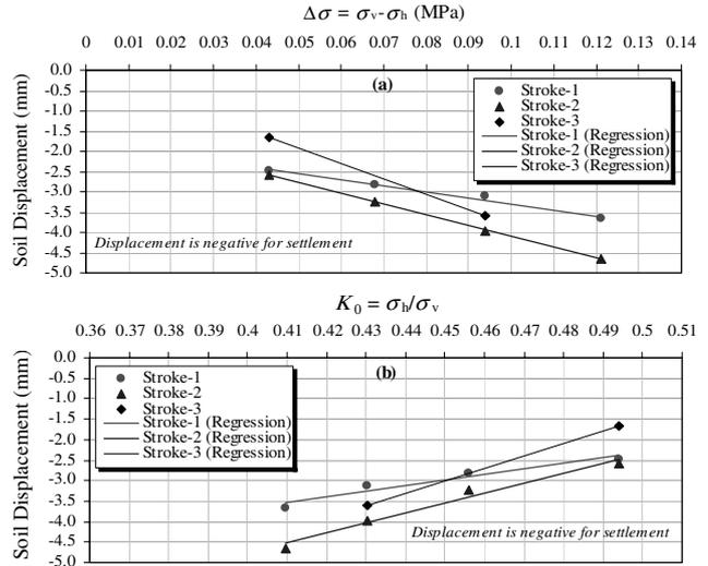
Figure 6. Variation of vertical displacement of soil surface with initial stress state: (a) stress difference  $\Delta\sigma$ , (b) stress ratio  $K_0$ .
