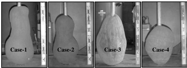
Figure 4. Shapes of injected grout bulbs.
