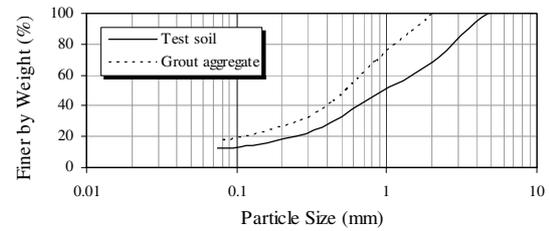
Figure 2. Gradations of test soil and aggregate of grout.
