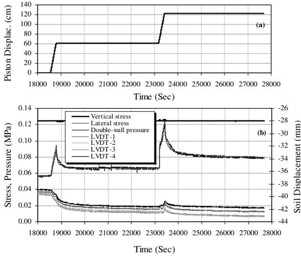
Figure 3. Injection results of Case-2: (a) pump piston displacement; (b) vertical displacement and stresses of soil.
