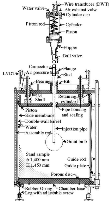
Figure 1. Setup of calibration chamber and injection pump.
