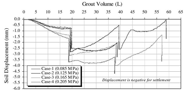
Figure 5. Vertical displacement of soil surface with injection.
