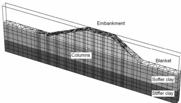
Figure 9. Overview of the 3D finite element model.
