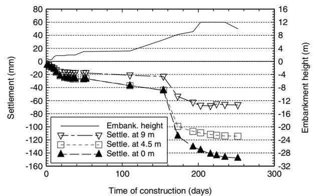
Figure 8. Settlements measured by the extensometer.
