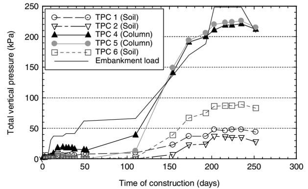
Figure 7. Total vertical pressures measured.
