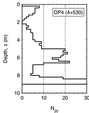
Figure 2. A typical dynamic penetration test in the area.
