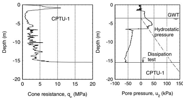
Figure 3. Static penetration test (“piezocone”).
