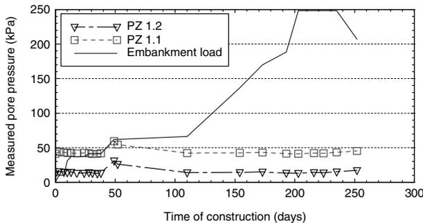
Figure 6. Measured pore pressures.
