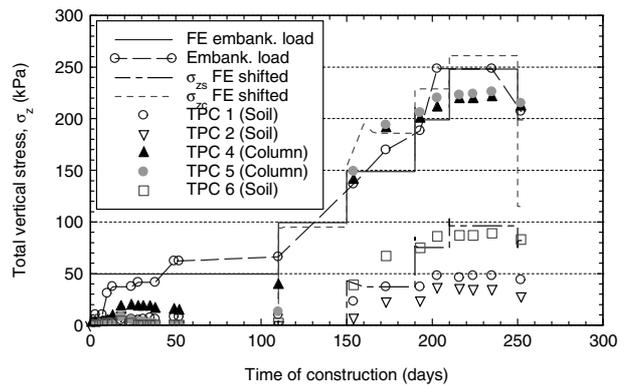
Figure 11. Total vertical stress comparison.
