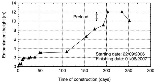
Figure 5. Embankment elevation rate.
